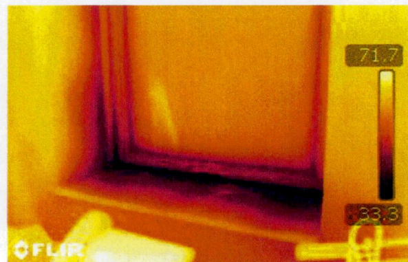
Figure 4: Close-up thermographic image shows cold air infiltration occurring around a window (typical).
