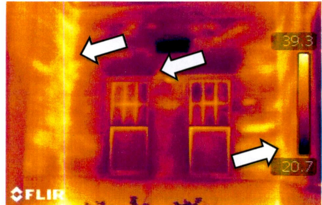
Figure 4: Exterior thermographic image indicates warm energy transfer at the inside corners and at the window perimeters.
