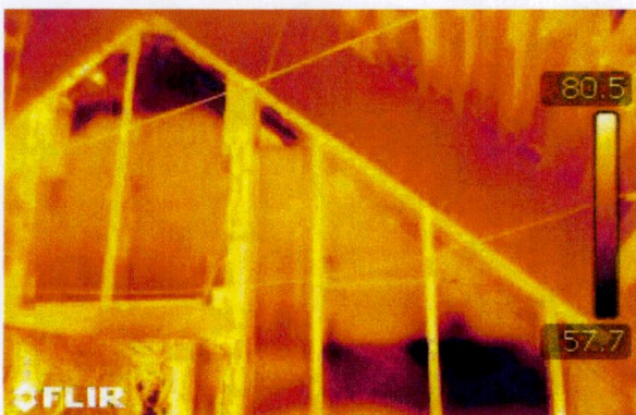
Figure 2: Thermographic image from inside the attic shows cold air infiltration at the gable wall transition to the roof ridge.
