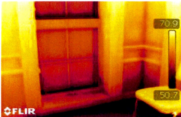
Figure 5: Thermographic image from inside Room 202 shows cold air infiltration in the wall at an outside corner and at the floor.
