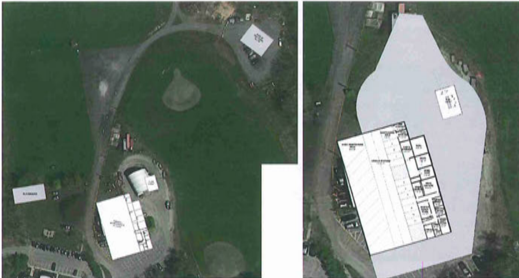
DPW Option 1: Replace in-place. Site blocking sketch and floor plan layout show lack of space on the site for salt barn, visitor/staff parking, and vehicle movements.
