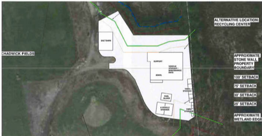
Option 4, Recycle Center: Site blocking sketch shows site layout constraints from the adjacent Johnson Field (lower-middle) and wetland setback boundaries which are depicted by red, orange, and green lines. These constraints forced an awkward layout that results in poor site circulation.
