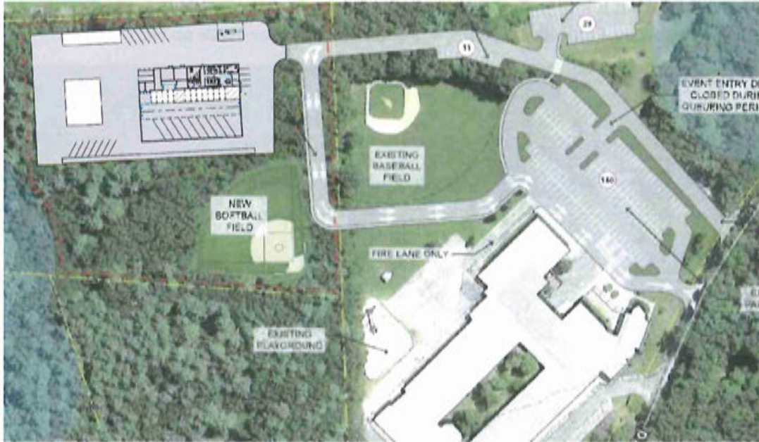
Option 3, Area 4: Site blocking sketch shows appropriate area for all program requirements and DPW site access connected to the Spofford Pond School. Alternative site access would connect to the DPW from the top left corner of the diagram above.
