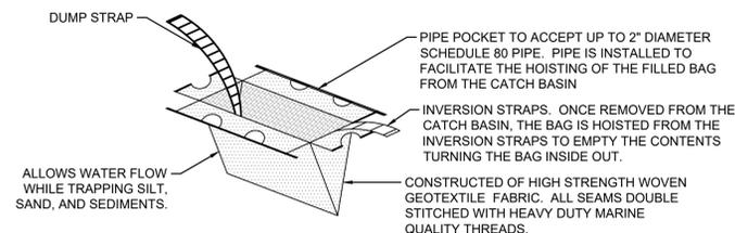
**GEOTEXTILE FABRIC INLET PROTECTION**
