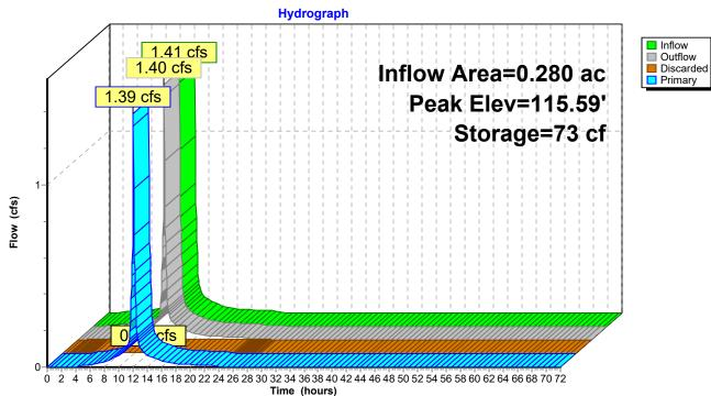
Time span=0.00-72.00 hrs, dt=0.05 hrs, 1441 points Runoff by SCS TR-20 method, UH=SCS, Weighted-CN Reach routing by Stor-Ind+Trans method - Pond routing by Stor-Ind method
