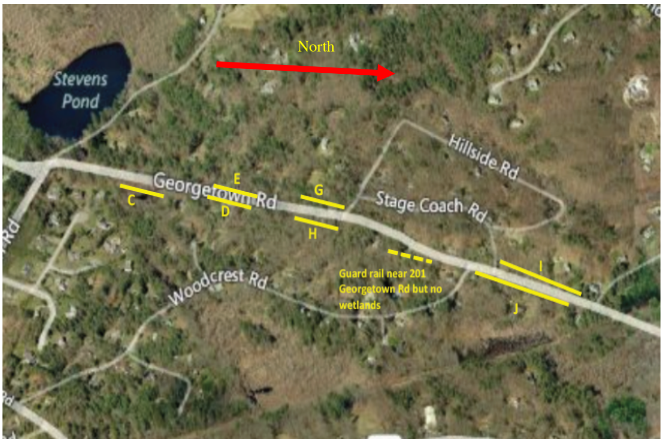
Figure 1. Georgetown Road just north of Ipswich Road where 8 guardrails are proposed for replacement. The various flagged wetlands (in letters) located below the guardrails are also shown.
