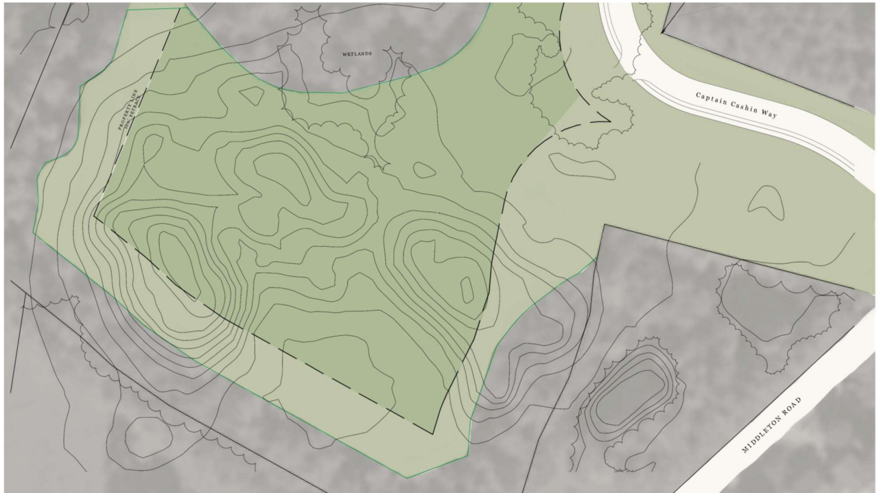
FIGURE 4: SCHEMATIC CLOSE UP OF THE BUILDABLE AREA OF THE COMMUNITY HOUSING AREA SHOWING THE 100 FOOT SETBACK TO PROPERTY LINES
