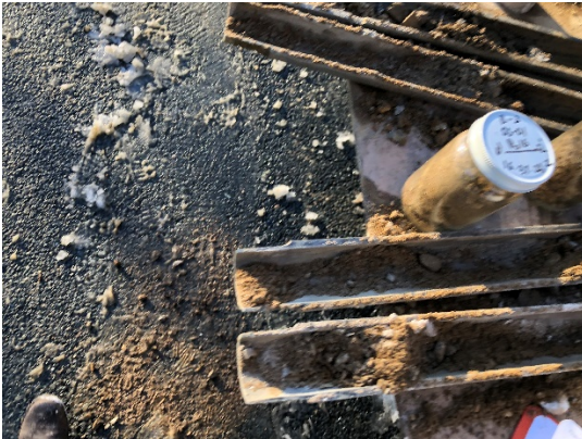
Silty Sand (SM) with Gravel (0' - 2')
