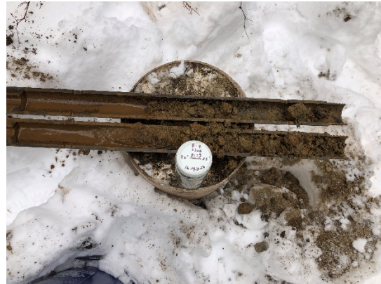
Silty Sand (SM) with Gravel (20' - 22')
